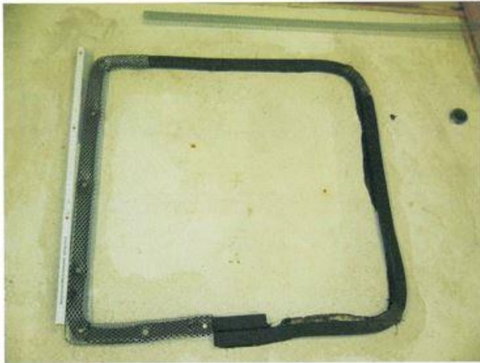
Fig.A2: Specimen with fitted swelling tape
